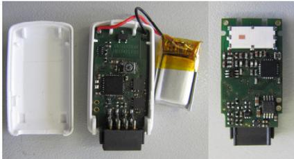
Above: Both sides of Microstim's 2-gram circuit board and its 1.6-gram battery. The white rectangle at the top right is the internal radio antenna.
