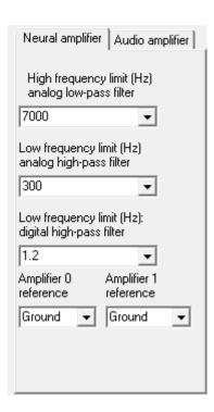
This panel allows you to control the analog low-pass and high-pass filters of the preamplifiers, as well as the electrode source of the analog signal reference.
