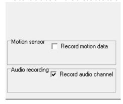
When using a logger that uses "flat" format, the control will appear as shown below. Note that ultrasonic audio recording is not supported by the flat file format.
