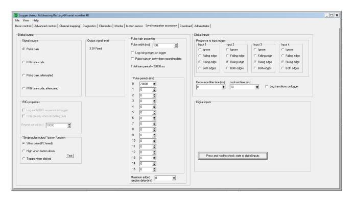
This tab is divided into two halves. The left panel controls the digital output while the right panel relates to the four digital inputs.
