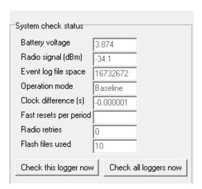
This panel shows the results of the most recent system check. This is a check of 8 important parameters of the system. You can initiate such a check by pressing "Check this logger now", or you can schedule automatic system checks by using the "System check options" panel of the "Advanced controls" tab. (See section 1.4.1). You can also chose which parameters to include in a system check using the "System Check Options" panel of the "Advanced Controls" tab.
