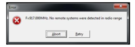
If no logger is switched on, switch it on, wait a few seconds, until its LED flashes red at a regular rate and press "Retry".
