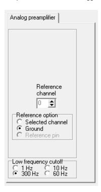
Select a suitable low-frequency cutoff (high-pass filter) using this control. Note that the analog filters here are first-order filters, so the cutoff is not particularly sharp. When in doubt, or close to the limit of a filter it is advisable to select a broader bandwith. For example, if signals around 70Hz may be of interest, it would be better to choose the 10Hz setting rather than the 60Hz setting.
