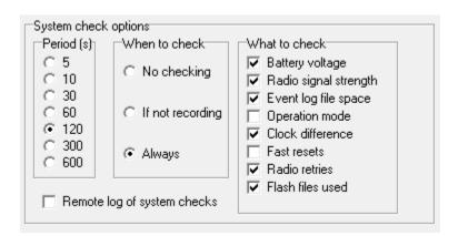
This panel allows you to control when the general system checks are conducted, and which of the parameters are included in these checks. If the "Remote log of System Checks" box is checked, then the results of each check will be recorded as a text string in the logger as well as the local log. The format of such a string is, for example, as follows:
