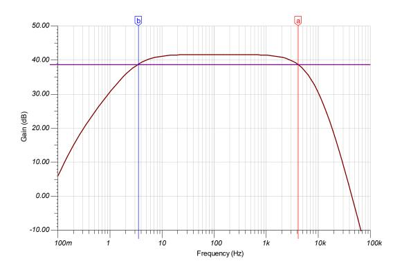
The total broadband input-referred noise is  $1.02\mu$ V rms. The total input-referred noise, when bandwidth-limited to 4kHz, is  $0.66\mu$ V rms. This represents a sensitivity that is better than the Intan preamplifier by a factor of 2.35, and a dynamic range that is greater than that of the Intan preamplifier by a factor of 4.6. The input-referred noise density at 1kHz is 10.63nV/rtHz.
