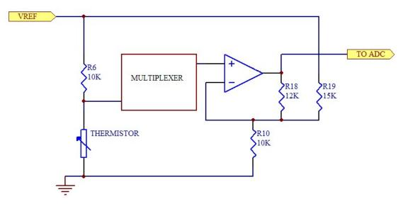
R6 and the thermistor form a simple voltage divider, so that the voltage fed to the multiplexer is given by
