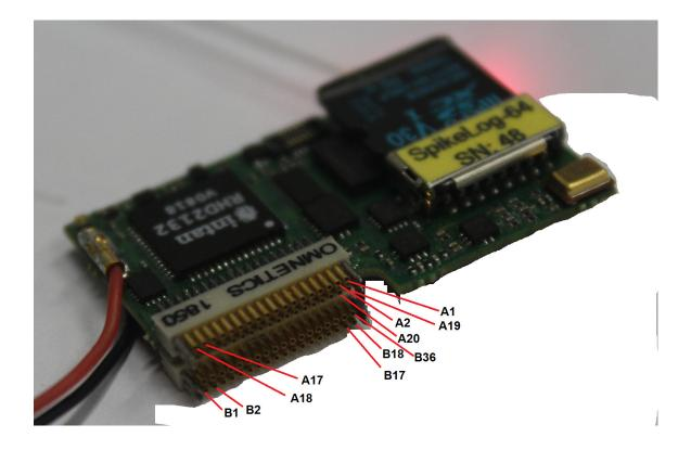
Each connector, A and B has 36 pins plus the steel support pins. The pin naming convention shown in the photo above is used so that if the logger is mounted rotated by 180 degrees, each pin of the A connector swaps function with the correspondingly numbered pin of the B connector. All 8 pins that are next to the support pins are GROUND. These are A1, A18, A19, A36, B1, B18, B19, B36.
